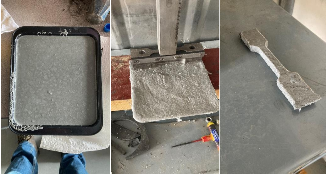
Fig. 1 Cookie cutter tensile specimen manufacturing method.
